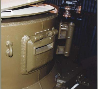
Above and left are a couple of photos I took of a preserved M3 Hybrid here in New Zealand that illustrate how things should look with the turret ring being vertical and recessed from the edge of the turret.
