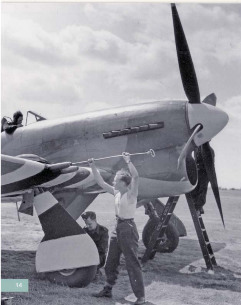
Left: armourers 'rodding' the original long-barrelled Hispano Mk II cannon which protruded from the leading edge of the wing on early Tempests.
