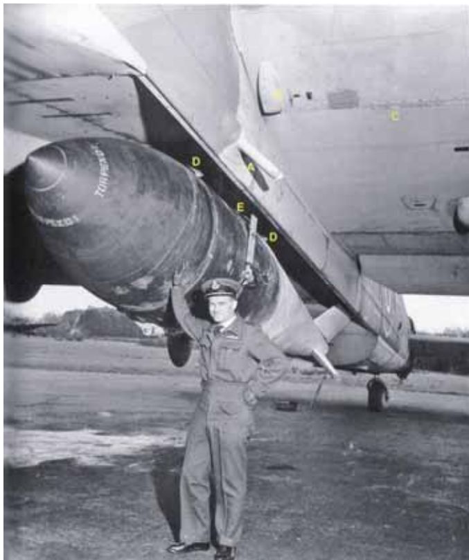
Left: 617 Squadron C.O. G/C Johnny Fauquier with his regular aircraft PD119 YZ-J. Of note are the trailing aerial shroud (A), cabin heating air exhaust vent (B) beneath the wing leading edge and main spar struts TIT JACKING PADS HERE (C). Below the rather crudely finished bomb bay fairings two adjustable bomb crutches (D) are visible, while resting on the Grand Slam are the electrical release and retraction cables (E). The Grand Slam itself has been noticeably marked by steel slinging cables during ground transportation. Below: A nice close-up of the restraint shackle underneath YZ-T PD113 (also seen on page 65). Normally electrically operated, the shackles' back-up mechanical release was a modified version of the glider and Upkeep manual release system, the operating T-handle being located on the pilot's floor forward of the flap lever. Visible here are the bomb release unit electrical cable (F), release unit ice guard (G) and manual release cable (H).
