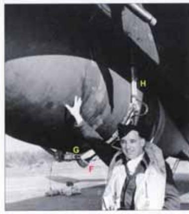
Left: 617 Squadron C.O. G/C Johnny Fauquier with his regular aircraft PD119 YZ-J. Of note are the trailing aerial shroud (A), cabin heating air exhaust vent (B) beneath the wing leading edge and main spar struts TIT JACKING PADS HERE (C). Below the rather crudely finished bomb bay fairings two adjustable bomb crutches (D) are visible, while resting on the Grand Slam are the electrical release and retraction cables (E). The Grand Slam itself has been noticeably marked by steel slinging cables during ground transportation. Below: A nice close-up of the restraint shackle underneath YZ-T PD113 (also seen on page 65). Normally electrically operated, the shackles' back-up mechanical release was a modified version of the glider and Upkeep manual release system, the operating T-handle being located on the pilot's floor forward of the flap lever. Visible here are the bomb release unit electrical cable (F), release unit ice guard (G) and manual release cable (H).
