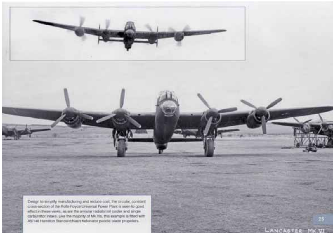
In order to facilitate service trials of the two-stage Merlin and Universal Power Plant (UPP) planned for the Avro Lincoln and Tudor airliner, commencing in late 1943 Rolls-Royce Hucknall installed UPPs in nine Lancaster Mk.IIIs, thus converting them to Mk.VIs. Although engine handling and servicing were found to be problematic, the Mk.VI showed a noticeable performance increase over a standard Lancaster. While some aircraft were retained for development work by Rolls, several Mk.VIs like JB675 seen here served on PFF squadrons.
