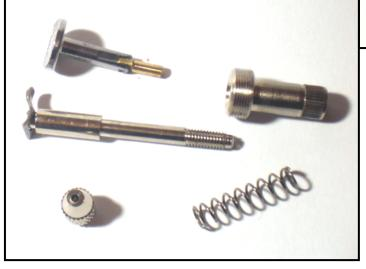
Once I looked inside the front end I was a bit disappointed. There was no complete head unit, just a 3-piece assembly that covered the nozzle. The nozzle mounting is like nothing I've seen before. It is actually a long brass tube protruding from a recessed area at the front of the main body. The nozzle itself is fairly standard but the whole thing left me with an impression that the aim was for cheapness of production rather than value for money.
