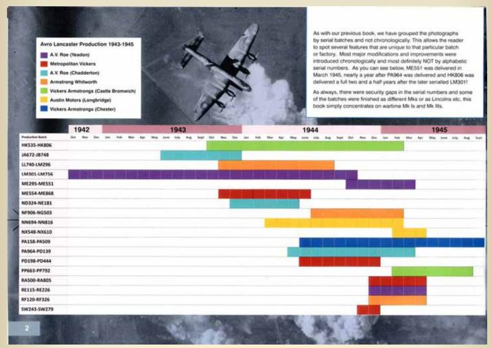
First up is a chart giving the production serial ranges and the factories that produced them. The following chapters begin to detail all the changes carried out, and the upgrades made to air-frames already in
