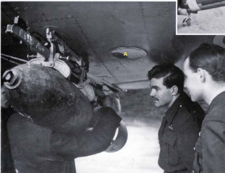
Bottom right: Armourers manoeuvring a 250lb bomb on to the port Mk.III Universal Bomb Carrier of P6971, in part of the sequence as the photo at left. The thin rods (B) are the bomb carrier sway braces.
