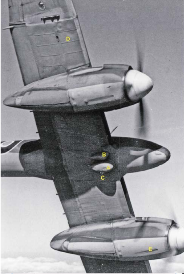
Right: Close-up of a Mk.III Universal Bomb Carrier fitted under the starboard wing of P7062, HE+L of 263 Squadron. Also of interest is the way the end of the nacelle folds over the rear of undercarriage bay.
