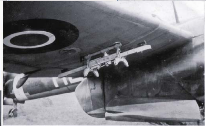
Left: A close up with lightened shadow areas, showing the positions of the cartridge case ejection box (A), the camera gun housing (B) and the downward identification lamp (C). The raised ribs over the wing fuselage tanks (D) are visible as are the oil stains (E) emitting from the small vents under the nacelles.
