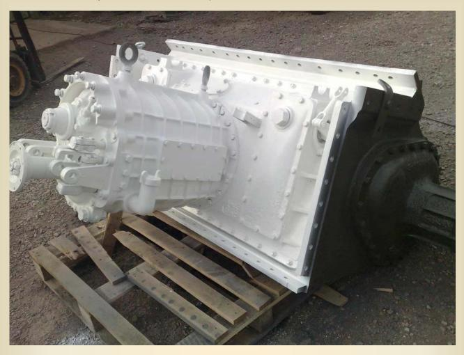
This assembly is the entire nose casting of the vehicle inside of which are the drive gears for the front sprockets, the brake assemblies, and the gearbox. The gearbox protrudes into the front compartment and divides the driver's and co-drivers positions.
