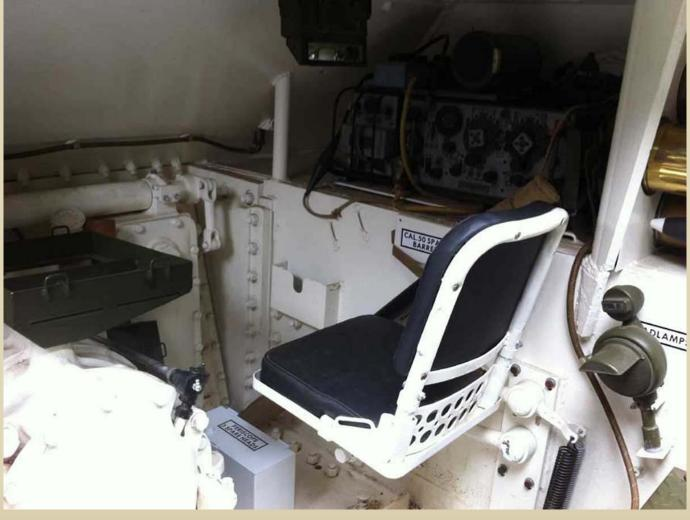
Note the position of the instrument panel and master switch on the left sponson, and the No.19 radio set on the right side. Note also how the seats were mounted on spring-loaded arms attached to the hull sides, not on a pedestal as were the standard Sherman seats. A better view of these mountings is shown in the photo below.
